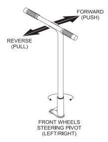
Figure 7. T-Handle (Directional Control)
